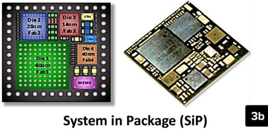
Figure 3: Heterogeneous integration takes various dies and discrete components and integrates them onto fine-line substrates (such as PCBs). (Source: IEEE HIR)
