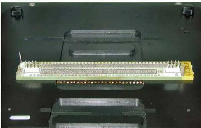
Figure 4: Close up of the bed of nails in the DELAM tester.
