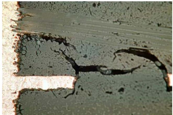
Figure 5: Cohesive crack.
