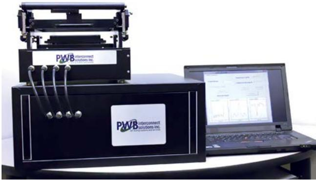
Figure 3: A DELAM tester.
